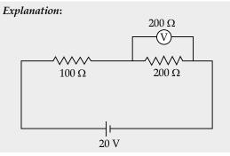
Voltmeter has resistance 200  $\Omega$ , which is connected across a 200  $\Omega$  resistance in parallel. So, the equivalent circuit is  $100 \Omega$  $100 \Omega$  $\underbrace{ \leftarrow V_1 \longrightarrow \leftarrow V_2 \longrightarrow}_{20 \text{ V}}$  $\frac{V_1}{V_2} = \frac{R_1}{R_2} = 1$  $V_1 + V_2 = 20$  $V_1 = V_2 = 10 \text{ V}$
