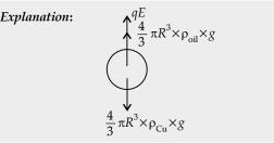
For equilibrium condition, net force acting in the particle must be zero. Hence,  $qE + F_B = mg$ Where symbols have their usual meanings. The buoyant force,  $F_B = \frac{3}{4}\pi R^3 \times \rho_{oil} \times g$  and weight  $mg = \frac{4}{3}\pi R^3 \times \rho_{Cu} \times g$ .  $q = \frac{4\pi R^3(\rho_{Cu} - \rho_{oil})}{3E}$   $= \frac{4\pi \times (0.5 \times 10^{-2})^3(8 - 0.8) \times 10^3}{600\pi}$  $= 2 \times 10^{-5} \text{ C}$
