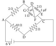
In steady state the current will flow through 1  $\Omega$ resistance as DF & DE becomes open. Now the circuit can be drawn like this:
