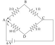
Let  $i_1$  current following in ABC and  $i_2$  in ADC line.  $R_{\rho}$  across ABC line is  $2 + 1 = 3 \Omega$
