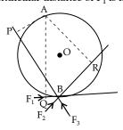
Perpendicular distance of  $F_1$  from A is AQ. Perpendicular distance of  $F_2$  from A is AR. Perpendicular distance of  $F_3$  from A is AP.
