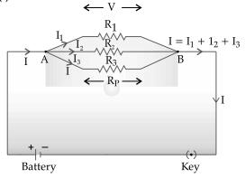
The given figure shows circuit consisting of three resistors  $R_1$ ,  $R_2$  and  $R_3$  connected I parallel.
