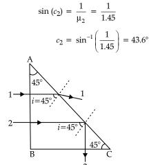
Ray '1' and '2' will fall on the side AC at an angle of incidence (i) of 45°. Critical angle of ray '1' is greater than *i*, so it will get refracted from the prism. Critical angle of ray '2' is less than that of *i*, so it will undergo total internal reflection.
