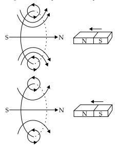
When the north pole of a bar magnet is pushed towards the coil, the amount of magnetic flux linked with the coil increase. Current is reduced in the coil from a direction such that it opposes the increase in magnetic flux. This is possible only when the current induced in the coil is in anti-clockwise direction, with respect to an observer. The magnetic moment M associated with this induced emf has north polarity, towards the north pole of the approaching bar magnet.
