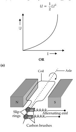
It works on the process of electromagnetic induction, i.e., when a coil rotates continuously in a magnetic field, the effective area of the coil, linked (normally) with the magnetic field lines, changes continuously with time. This variation of magnetic flux with time results in the production of a (alternating) emf in the coil.
