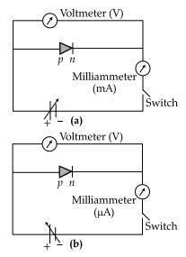
Using the circuit arrangements shown in fig (a) and fig (b), we study the variation of current with applied voltage to obtain the V-I characteristics shown below.
