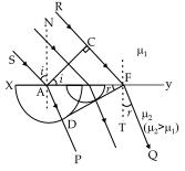
When point C of the wavefront in medium 1 traverses CF distance by that time (*t*) the wavelet from point A traverses AD distance. If  $v_1$  and  $v_2$  are the speeds of light in medium 1 and 2 respectively, then  $AD = v_2 t$  and  $CF = v_1 t$ .
