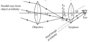
In an astronomical telescope there are two lenses – objective (O) and Eyepiece (E).
