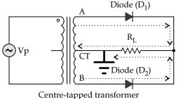
A centre-tapped transformer and two p-n junction diodes are used for a full weave rectifier.
