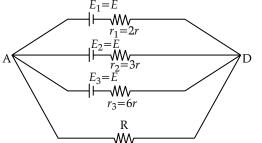
Current through cells (i) =  $\frac{E_{eq}}{r_{eq}} = \frac{E_1}{r_1} + \frac{E_2}{r_2} + \frac{E_3}{r_3}$ ...(i)
