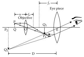
In a compound microscope there are two lenses – objective (O) and Eyepiece (E).
