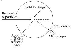
In the experiment, a gold foil of thickness  $2.1 \times 10^{-7}$ was bombarded by energetic  $\alpha$ -particles generated from <sub>83</sub>Bi<sup>214</sup> source.
