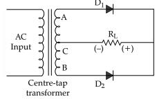
A centre tap transformer and two identical divides  $D_1$  and  $D_2$  are used to diagram a full wave rectifies. The centre-tap transformer has 3 output terminals. Centre tap is C is always at OV.
