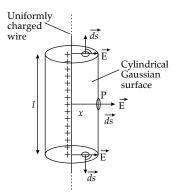
A cylindrical Gaussian surface of length *l* and radius *x* is considered with the wire as its axis.
