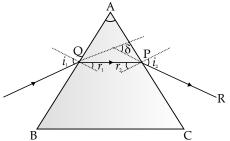
Angle of deviation  $= \delta = i_1 + i_2 + A$ Angle of prism  $= A = r_1 + r_2$
